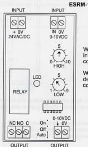
When the 0-10vdc input signal increases to the High setting contacts C-NO close.
